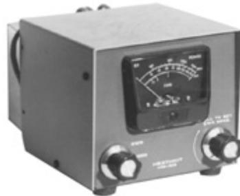
instrument measures both forward and reflected power, and it can be calibrated to measure VSWR.
