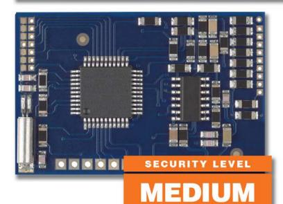
The SC20-455 scrambler offers medium level security for many brands and models of high frequency (HF) single sideband (SSB) radios. Transcrypt has designed the SC20-455's operating parameters to optimize performance for the HF SSB channel. The SC20-455 is a standard HF SSB scrambler for many military applications around the world, including the New Iraqi Army.
