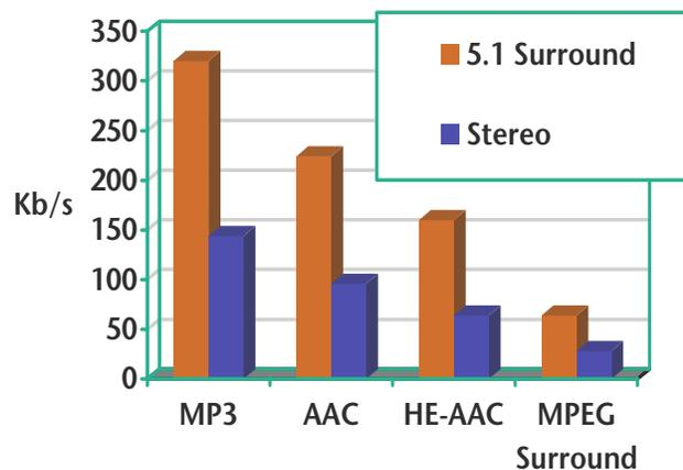
Figure 2. The evolution of MPEG Audio codecs has produced a 5 to 1 reduction in bitrate for similar perceived quality.
