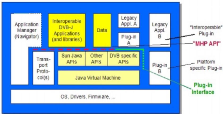
Figure 17. MHP reference architecture showing role of DVB-J
