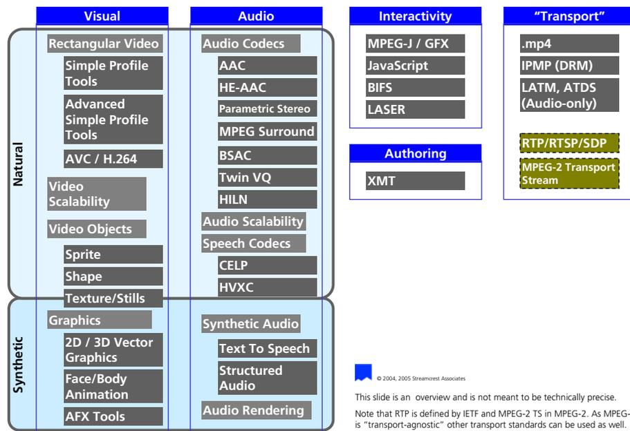
Figure 13. This is merely one way to classify MPEG-4's toolset. Courtesy Streamcrest Associates.
