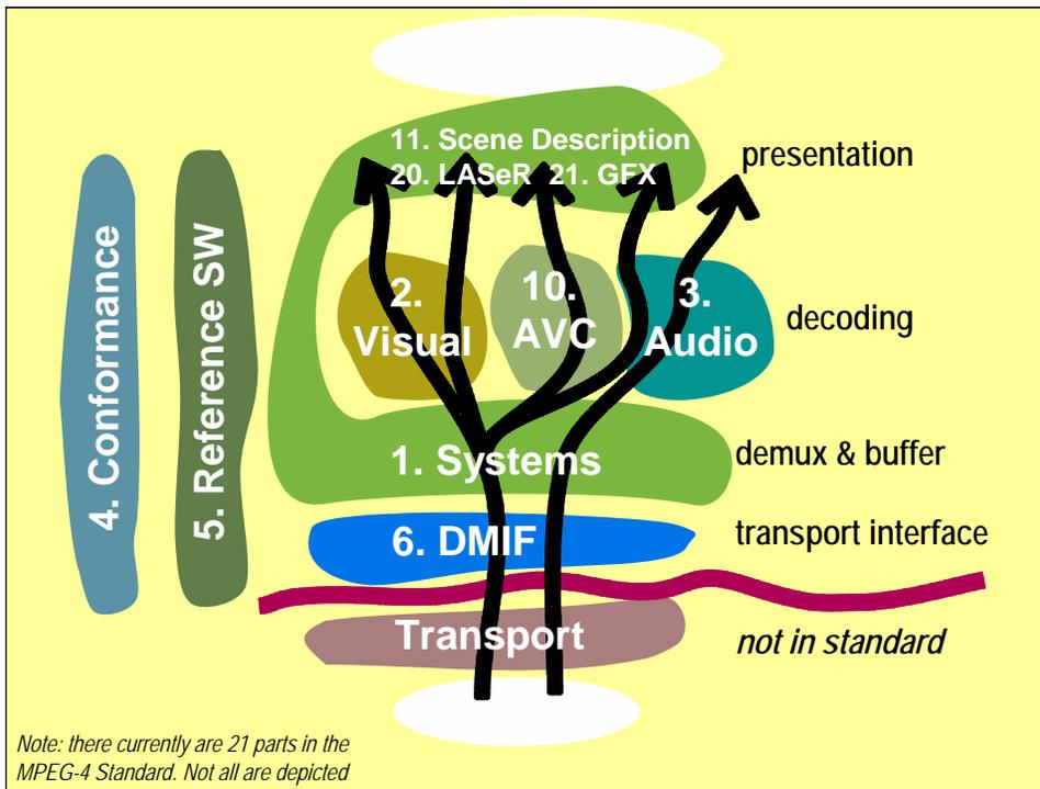
Figure 14. The parts of MPEG-4. The arrows represent the flow of bits through the MPEG-4 system.
