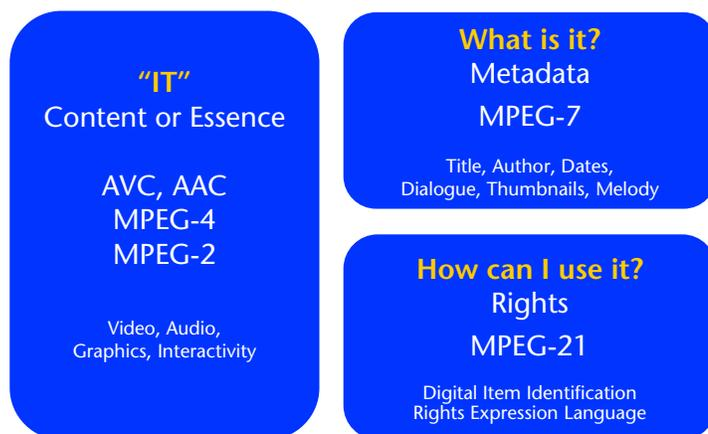
Figure 12. The Metadata and Rights Standards MPEG-7 and MPEG-21 are designed to complement coding standards MPEG-1, -2, and -4. Courtesy Streamcrest Associates.
