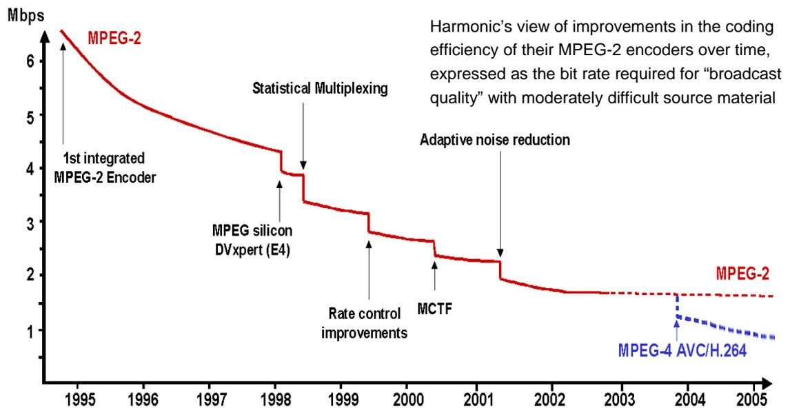
Figure 3. Improvements in coding efficiency are facilitated by MPEG-based competition. Courtesy Harmonic.
