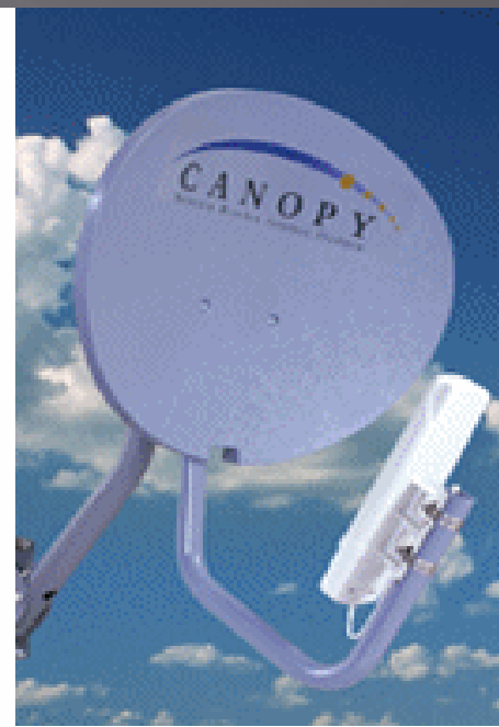
Backhaul Unit (BH)
